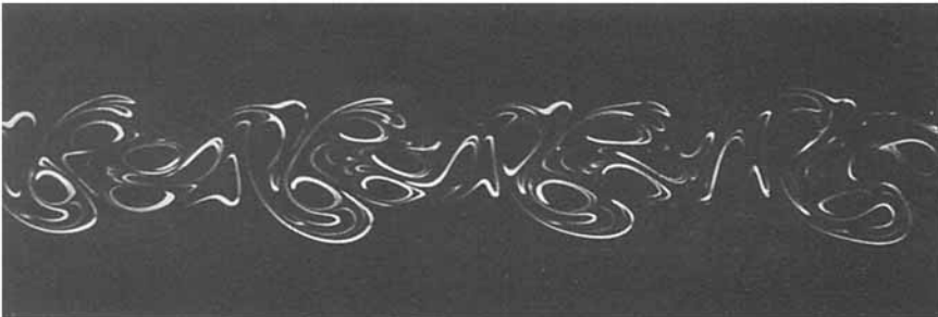
FIGURE 16. Flow visualization of quasi-periodic flow: f_1 = 3.5 Hz, f_2 = 4.9 Hz (flow is from left to right).
