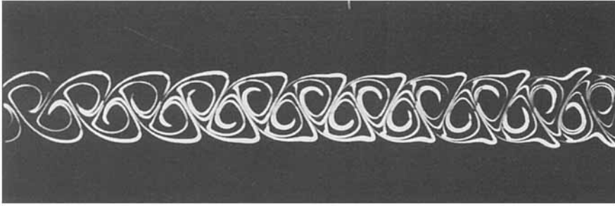
FIGURE 14. Flow visualization of locked flow: f_1 = 4.075 Hz = natural vortex shedding frequency (flow is from left to right).
